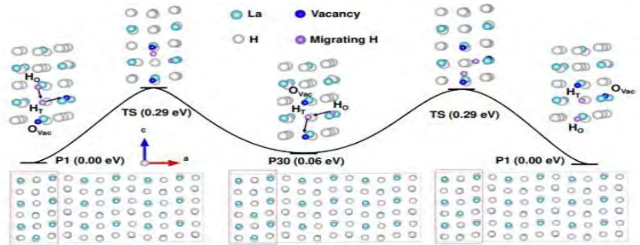
Schematic diagram of H ion transport path
