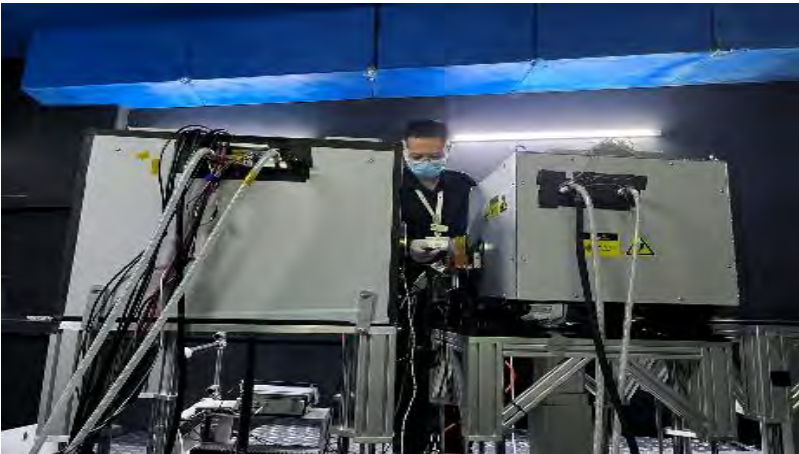
Multiple In-situ ^3\text{He} filter systems
