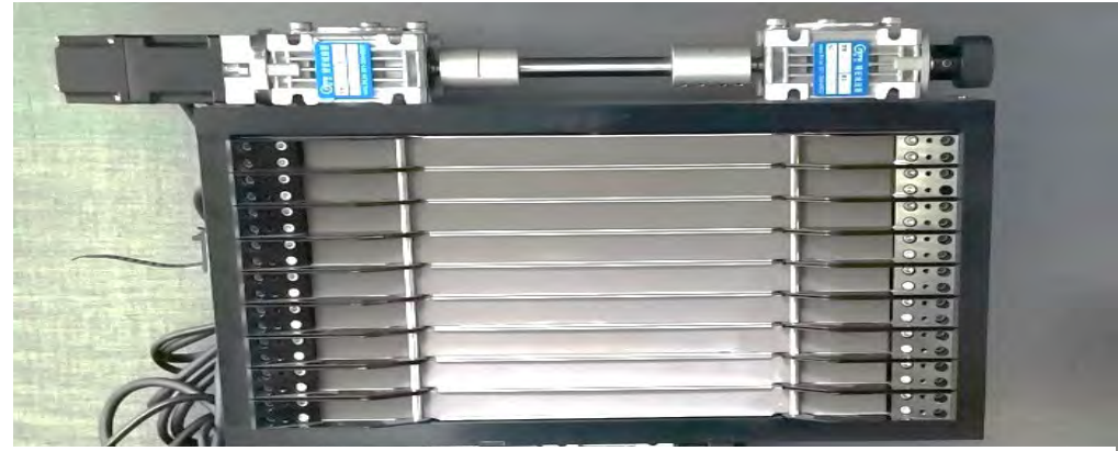
Double Focusing Silicon Monochromator applied in HIPD and RSD
