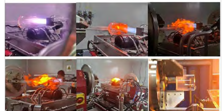
^3\text{He} cell fabrication
