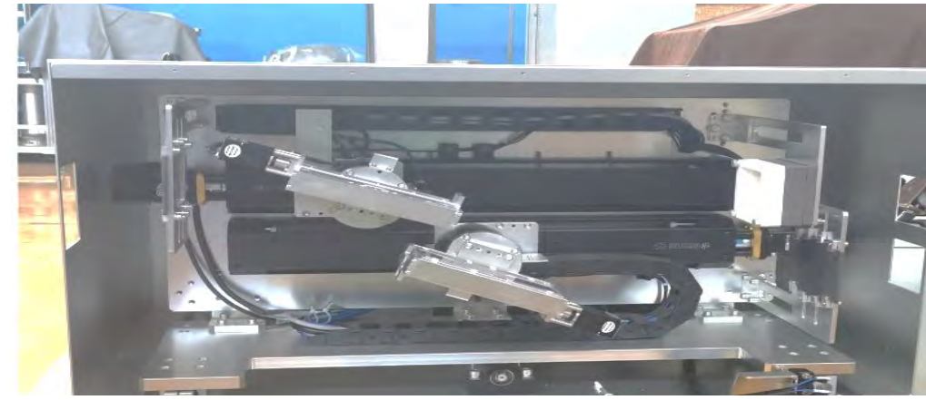
Double Crystal Graphite Monochromator applied in Cold Neutron Diffractometer
