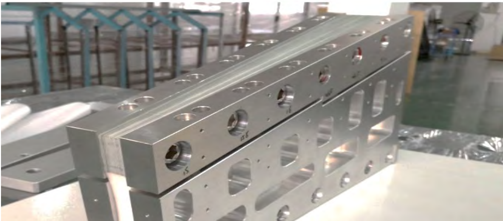
Neutron Radial Collimator applied in RSD
