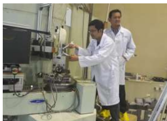
Fig. 3. Two PhD students from University of Indonesia performed residual stress measurements using Residual Stress Neutron Diffractometer
