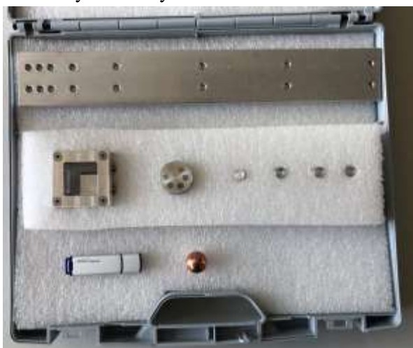
Fig. 1. IAEA Round-Robin sample to determine resolution of Neutron Radiography.
